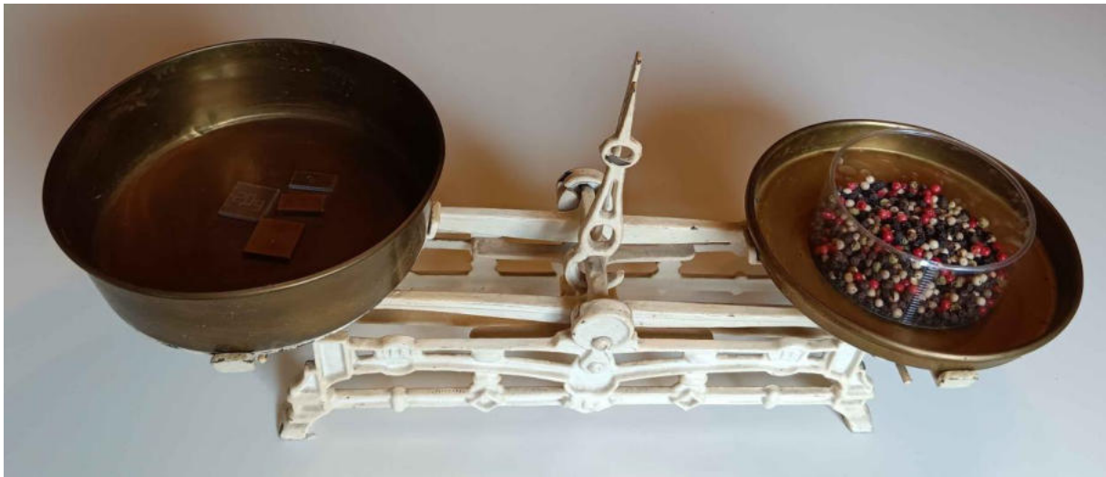
Fig. 19. The mass of a pile of mixed peppercorns is weighed on a Roberval balance with the proposed coin design. The balance equates the mass of the peppercorns to the mass of the coins. The mass of the coins is determined by adding the individual masses on the coins as 10\text{ g} + 5\text{ g} + 2\text{ g} + 1\text{ g} = 18\text{ g} . Therefore, the mass of the peppercorn pile is 18 g.
